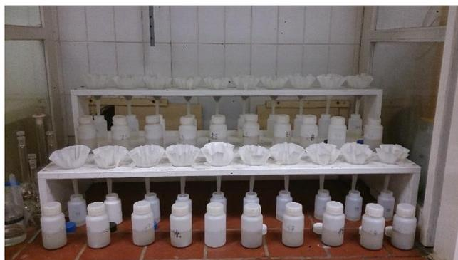
Figure 9: determination of carbonate content.
